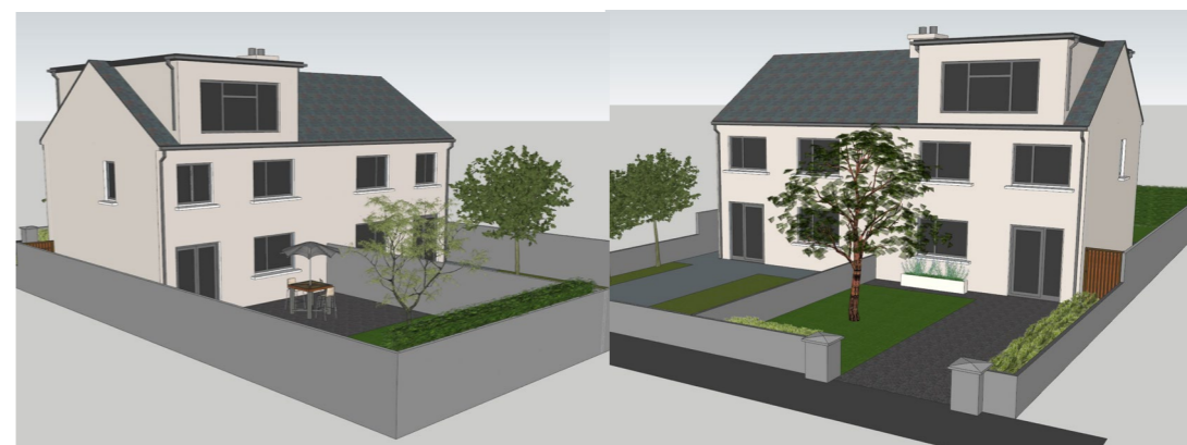
Figure 2: Poor Examples of Dormer Extensions
