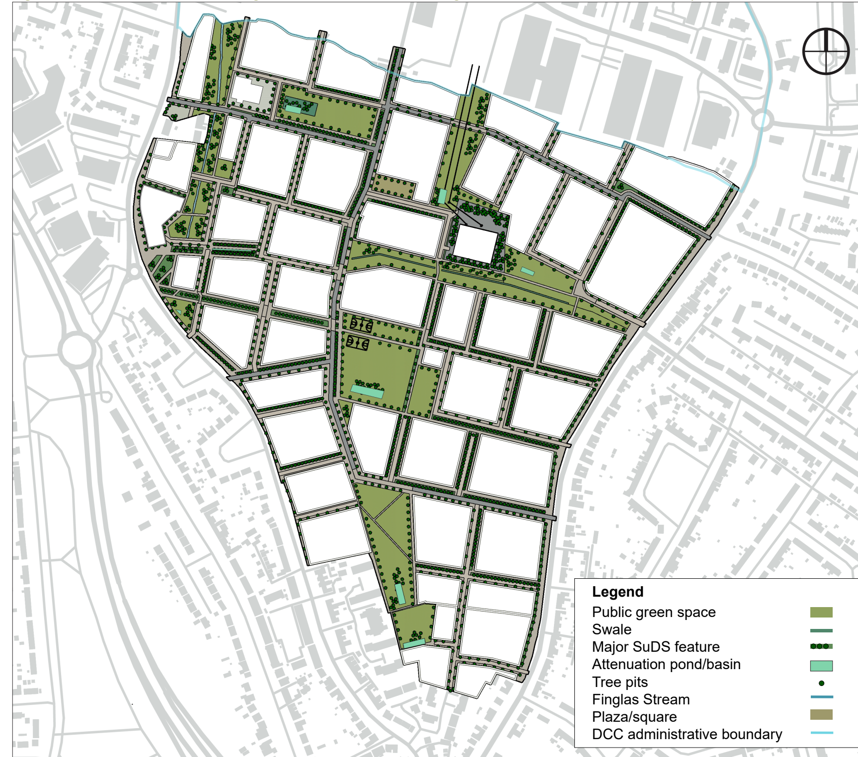
Figure 3.1: Sustainable Urban Drainage - Water sensitive urban design and nature based solutions concept
